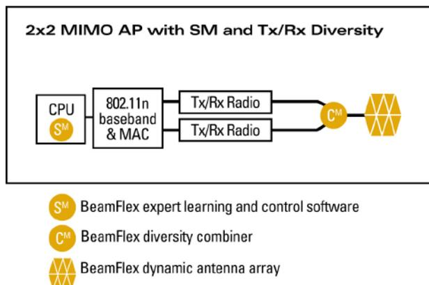
cost of a radio chain. By using a nimble, software-combinable antenna array to achieve diversity without additional radios and by leveraging commoditized, mass market Wi-Fi chipsets, BeamFlex produces performance and range optimization at a better price/performance ratio than pre-standard MIMO chipsets with multiple radios (figure 5, next page).
